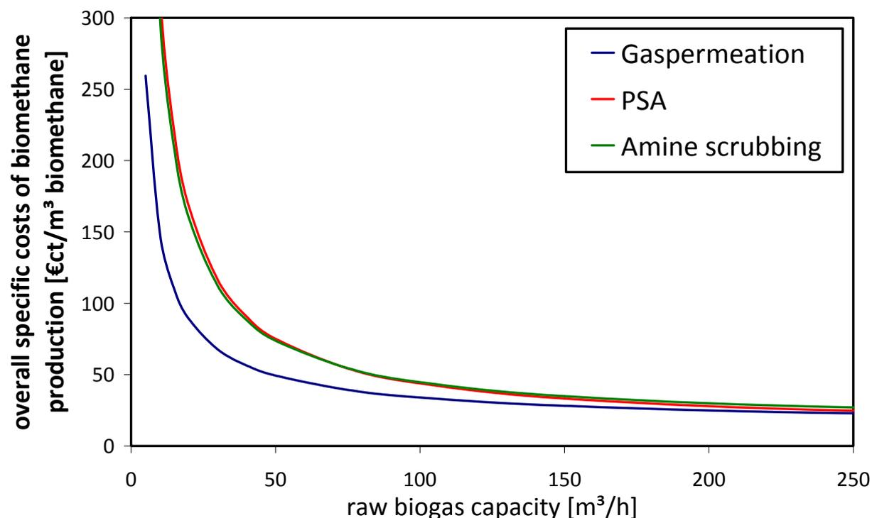
Figure 1: Economy of scale: degression of overall specific costs of biomethane production depending on raw biogas capacity for different biogas upgrading technologies
