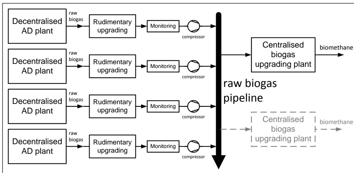
**Figure 9: Scheme of cooperative biomethane production using a concept of a raw biogas pipeline and a centralised biogas upgrading unit (even more than one biomethane production plant is conceivable); Source: Vienna University of Technology**
