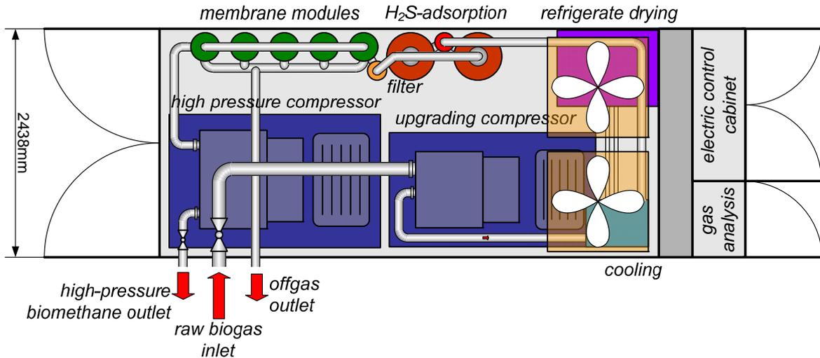
**Figure 3: Scheme of a mobile biogas upgrading unit with a capacity of 300m<sup>3</sup>/h raw biogas using gaspermeation mounted in a 20-foot standard container; Source: Vienna University of Technology**
