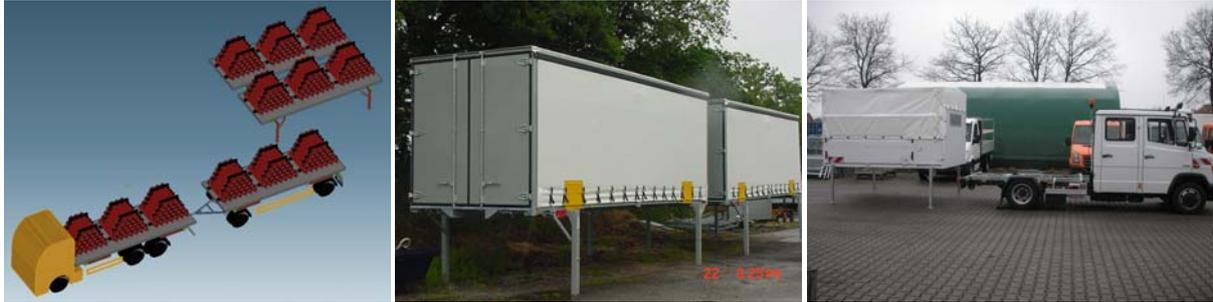
**Figure 6: Pressurised gas tank transportation systems applying WAB system: design study of gas transportation truck with 150 cylinders of 80 litres volume for 220 bar (left); swap trailer system (mid); light lorry with swap trailer body (right); Source: Güssing Energy Technologies GmbH, Schoon Fahrzeugsysteme**
